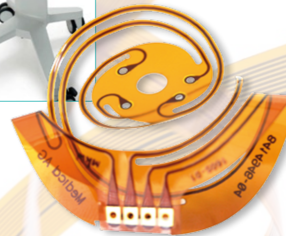
Flexible Leiterplatte zur Luftstrommessung Flexible printed circuit for air flow measurement
